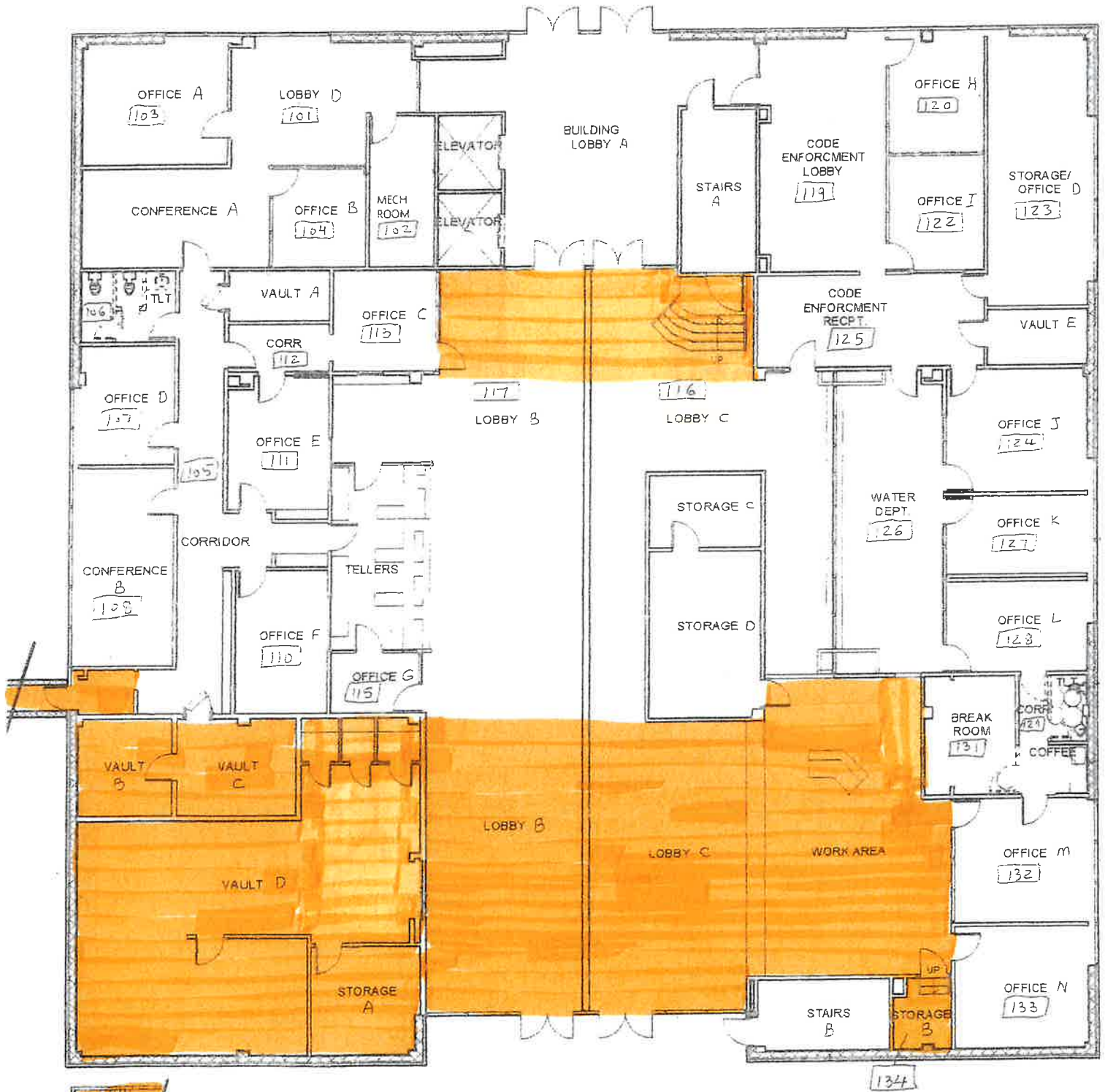
1 GROUND FLOOR DEMOLITION PLAN 1/8" = 1'-0"
